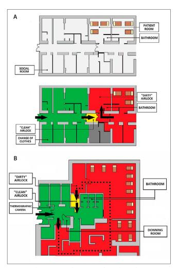
**Figure 6.** Work reorganization diagrams in two hospital exemplary units. A) Internal medicine department – view before (above) and after (below) reorganization. The airlock was created by placing walls across the corridor and excluding one of the patient rooms from use. B) Emergency Department – local conditions allowed the separation of entry and exit from the ward, introducing one-way traffic
